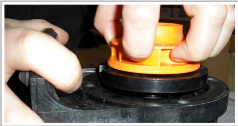
**Fig. 6b:** *Disassembly of impeller components*
