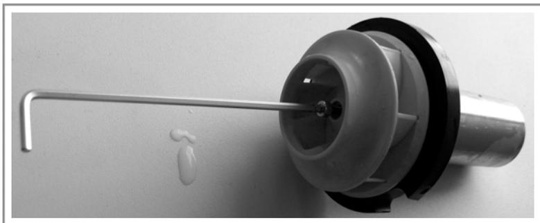
**Fig. 8: Disassembly of impeller wheel**
