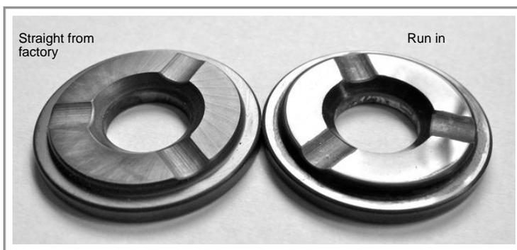
**Fig. 3: Bearing straight from factory and following run-in phase**
