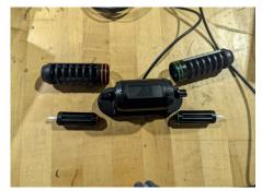
**Cleaning:** Once fully disassembled, place the propeller cages, propellers, and motor assembly in a 50/50 solution of hot water and vinegar, or a solution of citric acid for cleaning. This will ensure that the solution makes contact with the surface of each pieces, and ensure to remove any calcium build up on the axle and spindle.
