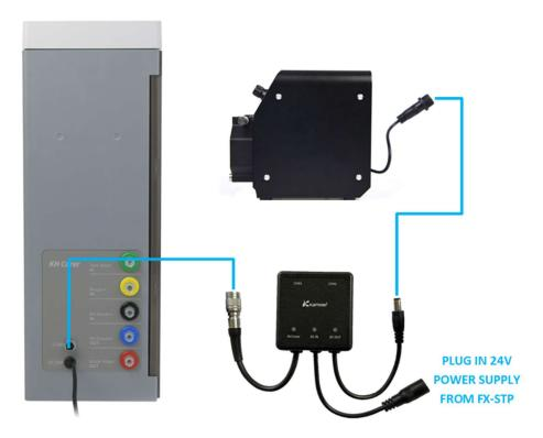
Connect the 'Click Lock' connector to the back of the KH Manager by aligning the locating ribs and pushing into place. **Excessive force must not be used when making the connection as it may damage the terminals.** To remove the connector at any time, pull back on the outer metal cover of the connector and it will slide back and release the connection.
