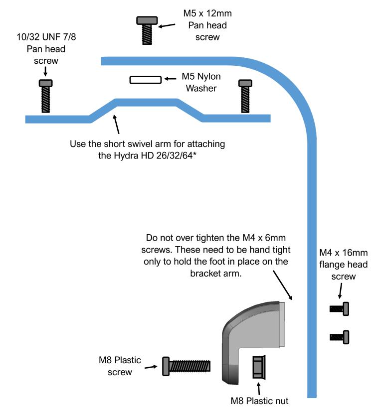
The M8 plastic nut should sit on the end of the screw against the aquarium glass to stop the plastic screw slipping.
