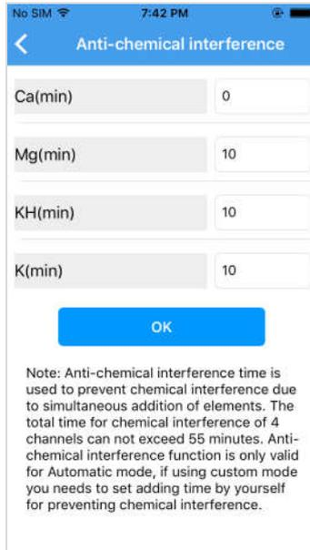
Anti-chemical interference time to add, prevent the element at the same time to add chemical interference, 4 channels of chemical interference cannot be more than 55 minutes, the chemical-resistant interference function is only valid for automatic mode, custom mode needs user to set the interval time to achieve the effect of chemical interference.
