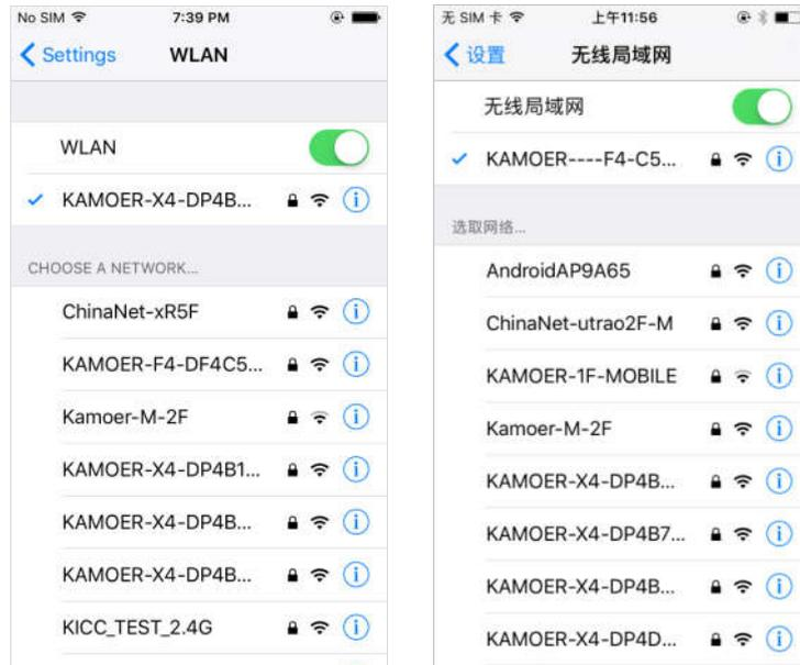
Step 2: Open the app, the dosing pump will be shown in the device list, click it to connect the dosing pump;
