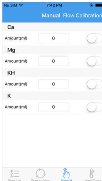
After setting the amount, turn on the right switch, the pump starts to run and stops automatically after the added amount is reached. If set to 0, turn on the switch then the pump will keep running, you need to turn off the switch to stop running.
