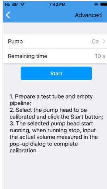
The purpose of the flow calibration is to improve the accuracy of the added element.
