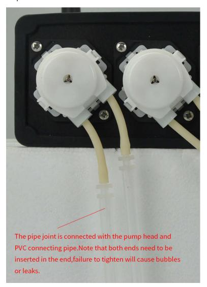
Step 3. The liquid outlet is fixed on the dosing pump tube rack.
