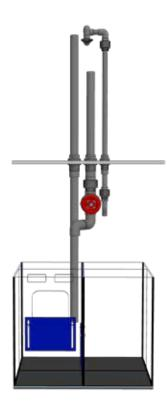
Return pipe: line up the top of the long pipe with the pre-fitted nozzle assembly on the weir.
