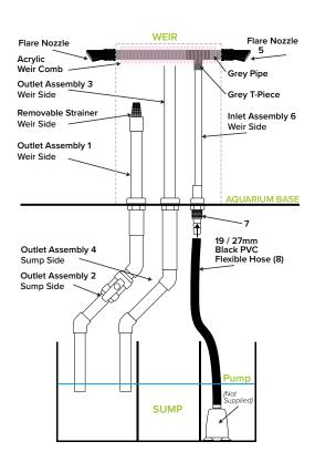
Please note when positioning the ends of the flare nozzles in the aquarium they must be kept close to the surface. Failure to do so may cause excessive water to be siphoned back into the sump and cause it to overflow in the event of a power outage.
