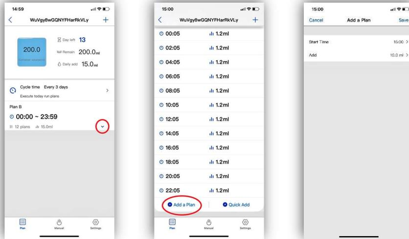
Plan groups and plan points can easily be deleted by swiping them to the left. When a plan point is deleted it will remove the volume of that dose from the overall group. The adjusted volume will be shown at the top of the pump page.
