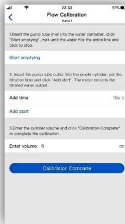
Please note the pump is only as accurate as the person completing the calibration. If high accuracy is needed it is recommended to use a measuring cylinder that can clearly read 0.05ml increments and is large enough to hold the volume of liquid produced in a full 60 second calibration run.
