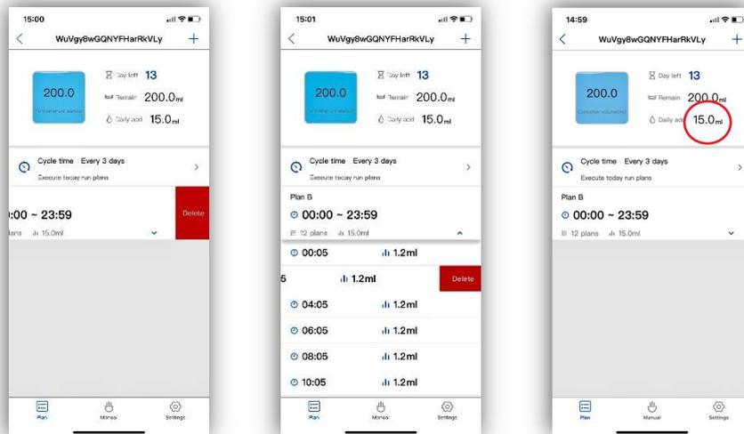
To reset all the plan points in a group, select the 'Quick add' tab associated with that plan group. The dosing amount, times and chemical interference can then be adjusted. Tap 'Save' to confirm the changes. Once saved any existing plan points for that group will be overwritten.
