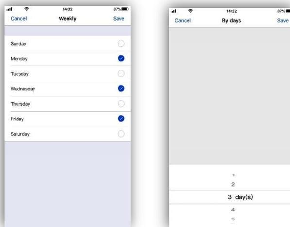
To set the dosing volume tap on the '+' button in the top right corner. Then set the name of the dosing plan and the time period to dose. It is factory set from 00:00 to 23:59 so that the dosing volume will be added throughout the full day, it can set to dose for a limited period e.g. between 10:00 and 18:00. Once the times have been set tap 'Save' in the top right corner.
