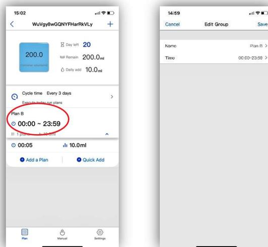
Plan points can be added to an existing group by selecting 'Add a plan' in the pump page. Enter the time for the additional plan point, the amount to be dosed and tap 'Save'. This will add to the total volume being dosed by that plan group and will be shown on the pump page. Any chemical interference set will be ignored by this point. The number of plan points available for each group will be determined by the overall time set for that group.
