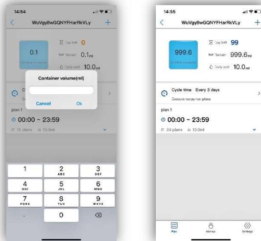
In the example below the pump has been set to dose every three days a total of 10ml, split into 24 doses, between 00:00 and 23:59. The dosing container has 999.6ml of solution left in it and should therefore last approximately 99 days.
