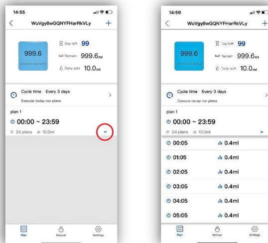
The time and volume of each individual plan point can be adjusted. Tap on the plan point and then adjust the time and dose amount as required, select 'Save' to confirm the change.
