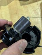
**NOTE:** If the bearing comes out of the motor with the impeller, this is totally fine and can be easily reinstalled using your fingers or something like a screwdriver. The bearing has a smooth side, and a side with two notches, always ensure the smooth side goes into the rubber gasket and the notched side points toward the impeller.
