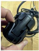
Removing the Impeller: Once the cage is removed, the impeller cover will be visible. Be careful when removing this piece, as there is a small bearing on the inside of the cap that has the potential to fall out, or stay on the front side of the impeller. Grab the cover by the inner diameter and carefully pull it out of the pump, you may need to shimmy this out as it is a tight fit. The impeller can then be removed from the internal shaft.
