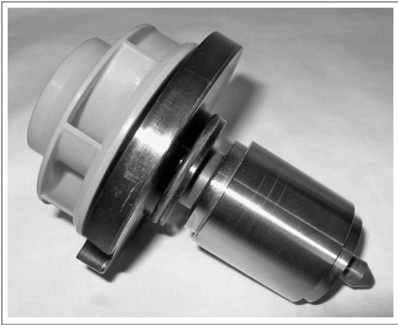
Fig. 7a/b: Removed impeller component, close-up of bearing (right)
