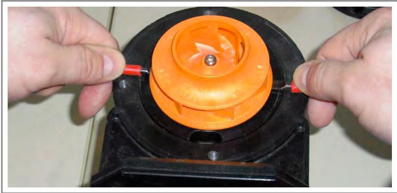
Fig. 6a: Loosening of impeller components
